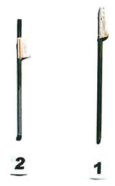
Rod #1 is coated with Rust-oleum®, Rod #2 is coated with Rust Bullet®
